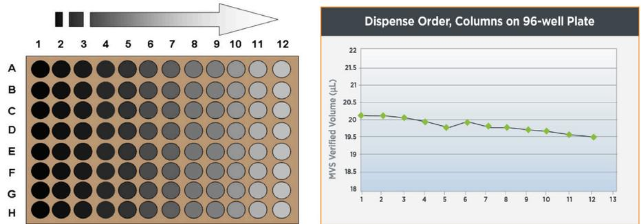
A schematic representation of a 96-well microtiter plate showing volume dispense trending. In this representation, an 8-channel device was used to dispense 20 µL across the plate from column 1 to column 12 (left). Although the volumes in each column should be identical, the actual volume is sequentially lowering (drifting downward) with each dispense (right).
