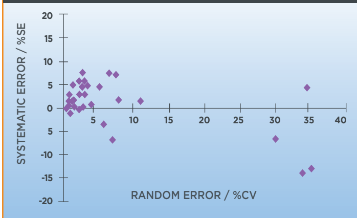
Figure 1. Pipetting skills assessment of fifty-three QC technologists prior to receiving pipetting technique training, dispensing 10 \mu L aliquots of sample (n=5) using the same calibrated pipette.
