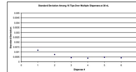
Figure 5. Standard deviation among 16 tips over multiple uses
