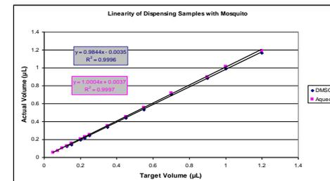
Figure 6. Volume Transfer Linearity of mosquito
