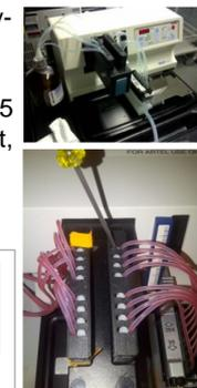
**Figure 2.** The WellMate can be optimized tip-by-tip by adjusting the set-screws within the cartridge assembly.
