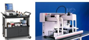
Figure 1. The ARTEL MVS® Multichannel Verification System (left) was used to assess the volume transfer performance for the Beckman Coulter Biomek FX (right) for the RT-PCR assay.
