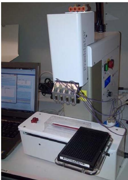
**Figure 1.** The 4-tip Preddator showing the MVS 384-w Verification Plate loaded on the plate deck before a volume transfer measurement. The reservoir trough, which is seen below the tips, was employed when priming the tips before the initial dispense. Tip ID #4 is the right-most tip and tip ID #1 is the left-most tip.
